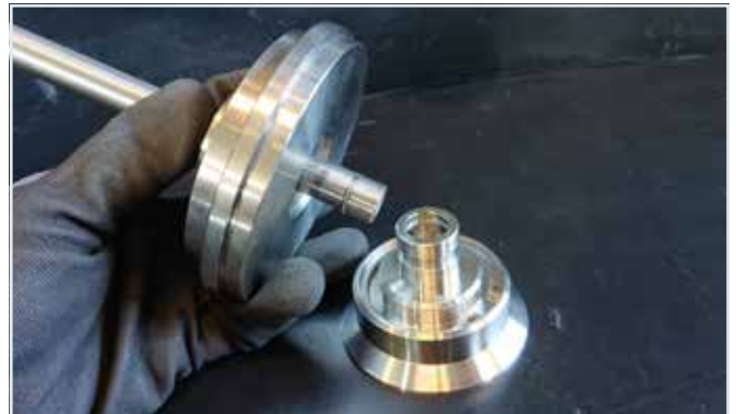
4.12 Insert spindle into disc. • DN 15 - DN 50 The spindle must engage in the groove of the disc with a round wire snap ring. • DN 65 – DN 100 Push the spring cotter pin sideways into the groove.
