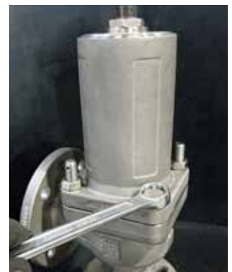
Screw connection of spring housing and body.
