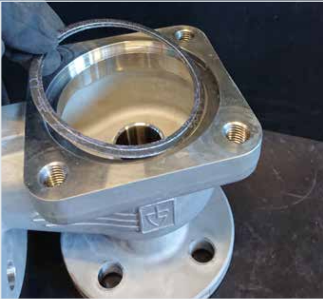
7.8 Place new graphite packings in the housing and welding plate.
