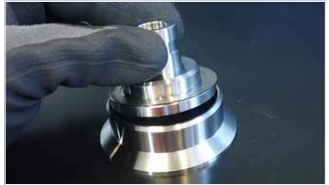
4.8 Insert disc and shim rings. 4.9 Secure with a new circlip.
