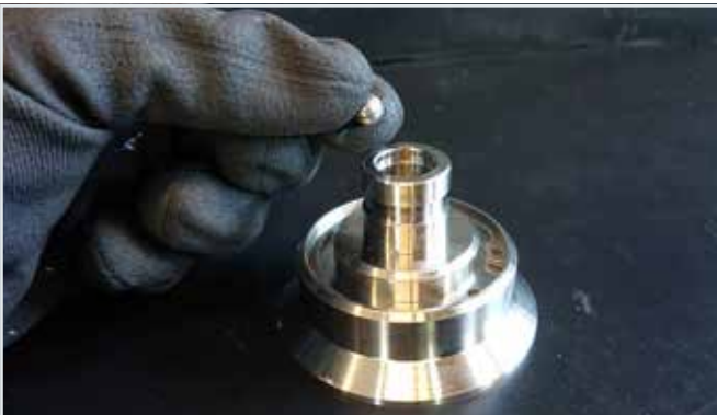
4.10 Bore bottom of disc with some stainless steel grease and insert the ball. 4.11 Coat the contact surface of spindle for ball with some stainless steel grease.
