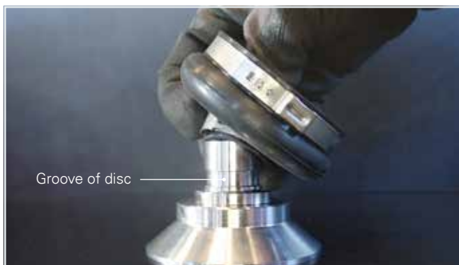
5.11 Place ear clamp in outer groove of elastomer bellows.
