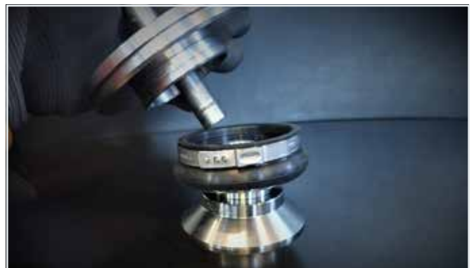
5.14 Coat the bottom of the bore of the disc with some stainless steel grease and insert the ball.
