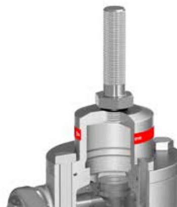
Figure 10: The spindle is free and the cap is sealed gas-tight
